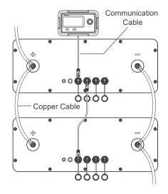
(not included). The Renogy Monitoring Screen or the Renogy Bluetooth Module should be connected to the RS485 UP Communication Port of the first battery.
